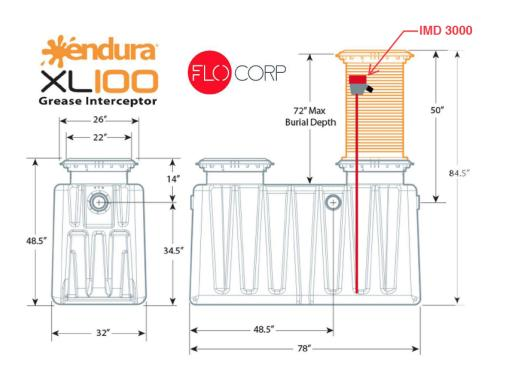
IMD 3000 has been calibrated to the interior characteristics i.e. corners and angles due to rotomolding of the fully recyclable HDPE high performance plastic used in manufacturing Endura XL100 Grease Interceptors.
