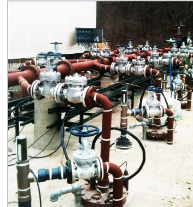
Figure 1. MEMFlo™ Volumetric Flow Meters in use during a fracking treatment in the Marcellus Shale.
