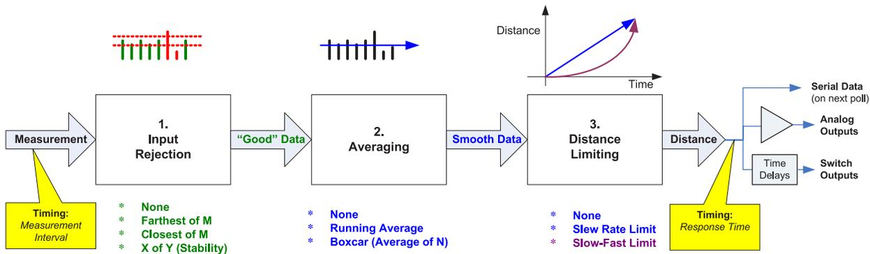
When using filters, the first valid measurement after power ON becomes the initial condition for all further processing. The Filter Options are shown in block diagram below, followed by a description of each.
