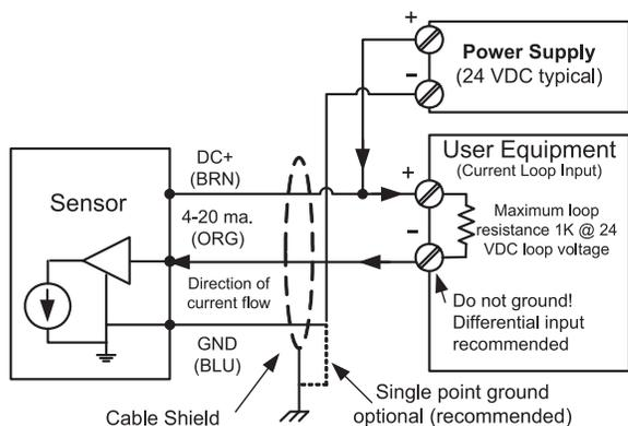
The default sinking loop output is a 4-20mA signal proportional to the measured distance between two endpoints set by the user. The current low/high values are Ranger Plus™ Software adjustable and match those of the sourcing loop. Current flows from the power supply through the user equipment then INTO the sensor (ORG wire).
