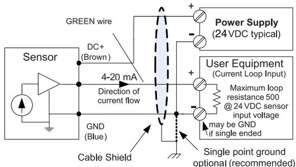
The default sourcing loop output is a 4-20mA signal proportional to the measured distance between two endpoints set by the user. The current low/high values are adjustable to any values between 0 and 20mA using Ranger Plus™ Software. The slope can increase or decrease with distance but all analog outputs must have the same slope. In a sourcing loop current flows out of the sensor, through the user equipment and back via the sensor's ground (BLUE wire).
