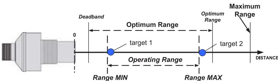
The sensor measures the distance to targets within the Operating Range (target 1 to target 2). This range can be set through the software by adjusting the Range MIN and Range MAX parameters. The factory default is the widest possible, deadband to maximum range.
