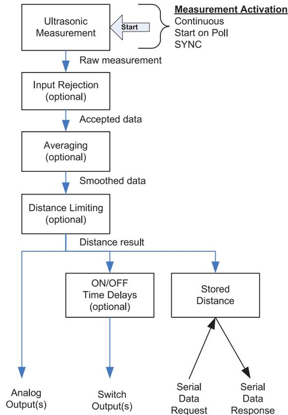
In Start on Poll activation the entire process is performed once per poll, i.e., M Input Rejection x N Averaging measurements. Some filters are disallowed in Start on Poll. If a poll is received before an ongoing measurement process finishes, the ongoing process will run to completion then another measurement process will begin.
