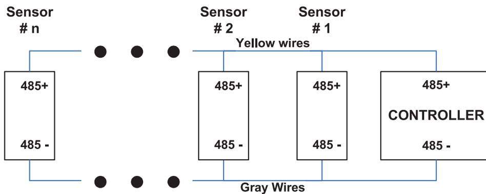
Before connecting to a network each sensor must be assigned a unique address and all sensors must be configured to the baud rate of the network controller, as described in following. The address assignments must also be different from other connected (non FLO-CORP) devices. Sensors used in a network must be configured in continuous or start-on-poll measurement activation depending on the needs of the system.
