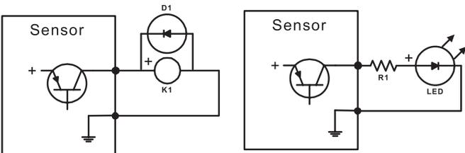
Switch ON energizes relay coil K1 -
