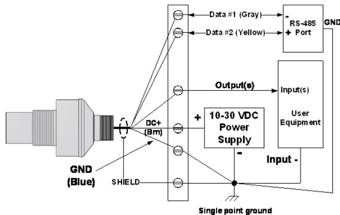
Up to 32 addressable sensors can be connected to the RS485 bus. Sensors can be configured into RS-485 addressable multi-drop networks as shown below.
