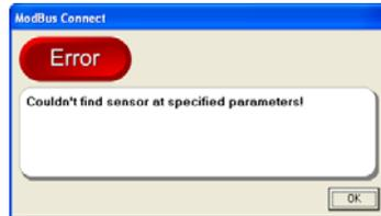
7. If the above error continues, use Find Sensor to scan all sensor interface combinations. The default is address is 1. Check the "All Ports" and/or "All Baud Rates" boxes if you are unsure of those. The software will identify the first Sensor Model found, starting at address 1 through 247. The window will appear as follows as the software searches for a sensor:
