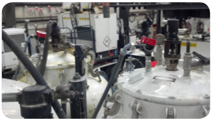
Fig. 2 shows the Tracer 1000 mounted in a small vessel where a minimum deadband was required. The Tracer 1000 3/4" NPT process connections was also required along with maximum accuracy and resolution.
