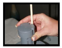
Reassemble the meter measuring tube by seating the O-Ring on the measuring tube first. Use a little lubricant on the O-Ring to facilitate reassembly. Using hands only, press the measuring tube firmly down into the meter body with a slight twisting motion. Replace the raceway, ball and clear scale tube. Replace the flange bolts but do not overtighten.
