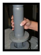
you want to read the scale. The notches are designed to give you a full 180° rotation. The guide rod and float assembly can be reassembled into the core tube.
