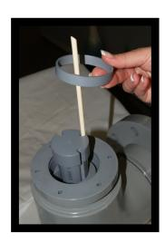
Reassemble the meter measuring tube by seating the O-Ring on the measuring tube first. Then use a little lubricant on the O-Ring to facilitate reassembly. Using hands only, press the measuring tube firmly down into the meter body with a slight twisting motion. Replace the raceway, ball and clear scale tube. Replace the flange bolts but do not over-tighten.
