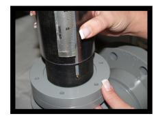
4) The float assembly includes 3 guide rod positions so the float assembly can be turned in the direction of the magnet that is encapsulated in the float assembly. The magnet position is indicated at the top of the float assembly with two indents at the top. The magnet should be aligned in the direction
