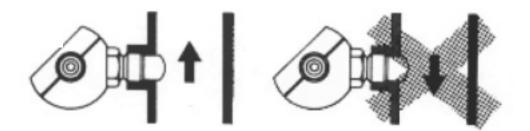
The unit is best installed on a horizontal line the best location to ensure constant liquid contact is the side of the pipe as opposed to the top where cavitation bubbles are more likely to exist.
